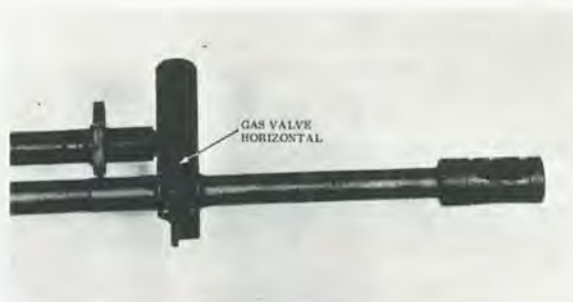
FIGURE 64. — Gas valve in horizontal position.
