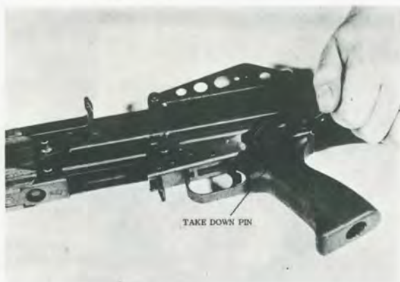
FIGURE 8. — Pushing out the take-down pin.
