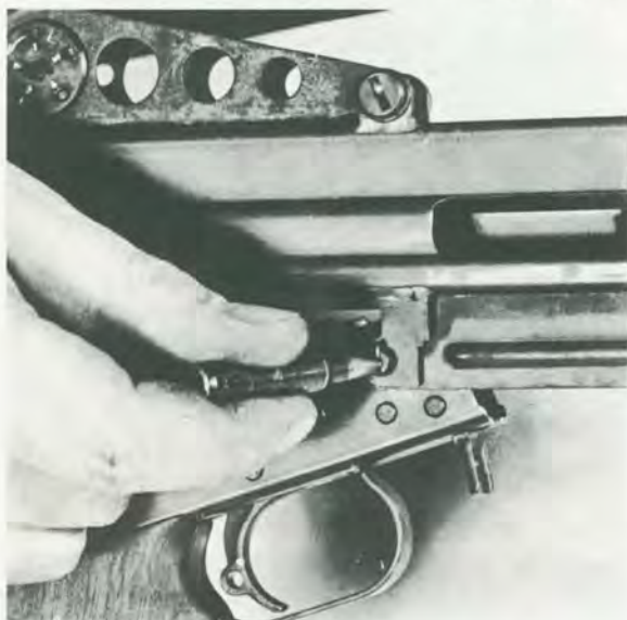
FIGURE 12. — Removing the trigger housing group retaining pin.
