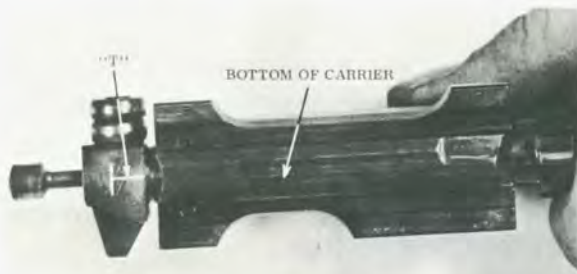
FIGURE 21. — "T" on carrier cap assembly in line with the bottom of the bolt carrier.
