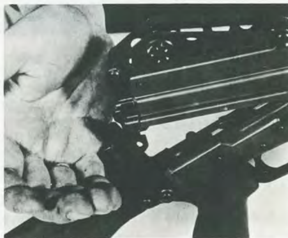
FIGURE 11. — Removing the carrier, piston and bolt assembly.
