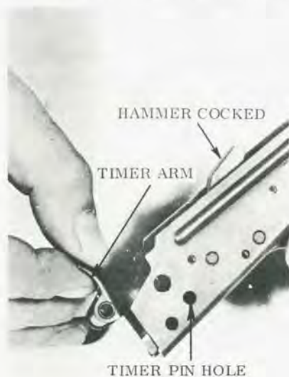
FIGURE 47. — Replacing the timer assembly.
