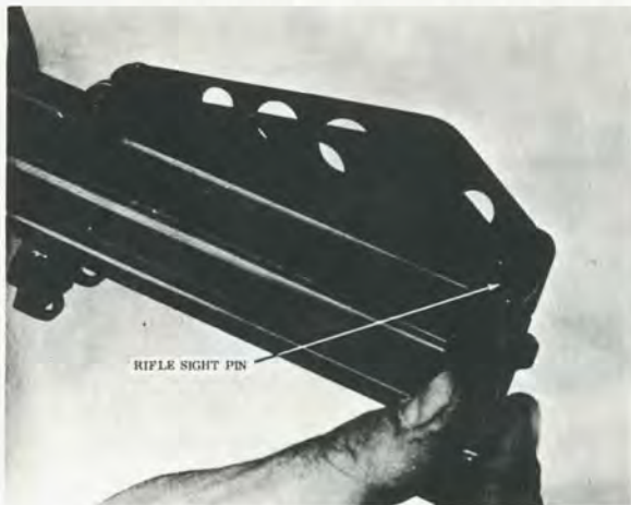
FIGURE 41. — Pushing out the rifle sight pin.
