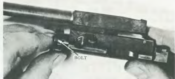
FIGURE 22. — Pushing bolt into carrier.
