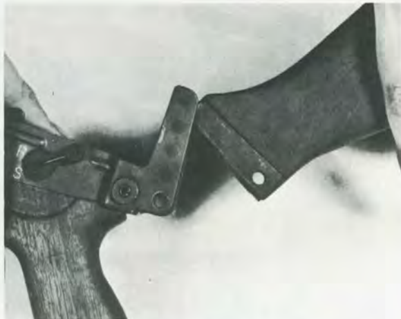
FIGURE 18. — Rotating the stock upward.
