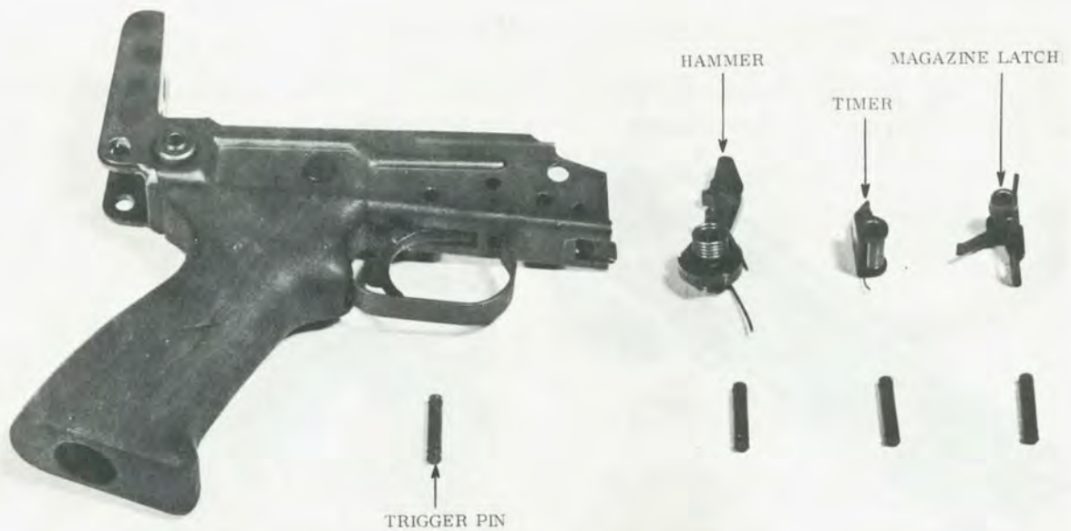
FIGURE 34. — Magazine latch, magazine latch pin, timer, timer pin, hammer, hammer pin, and trigger pin removed from the trigger housing group.
