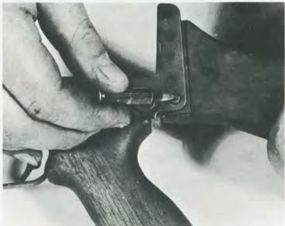
FIGURE 17. — Removing the stock retaining pin.
