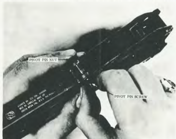
FIGURE 42. — Removing pivot pin and pivot pin screw.
