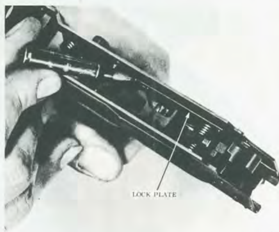
FIGURE 32. — Pushing the lock plate forward.
