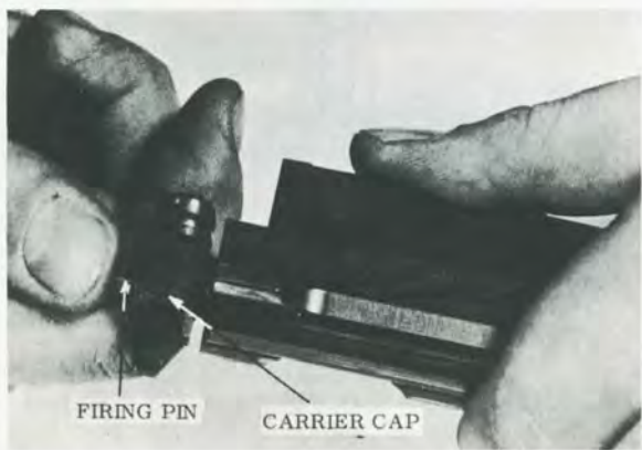
FIGURE 19. — Firing pin and back of the carrier cap assembly.
