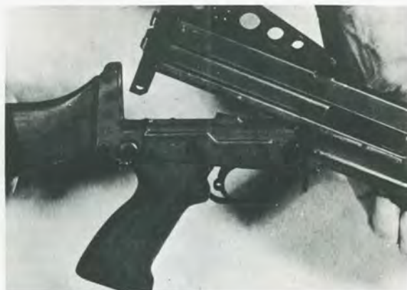
FIGURE 9. — Trigger housing group pivoted downward.
