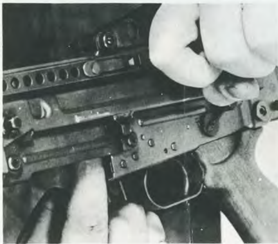
FIGURE 6. — Pushing up bolt stop.
