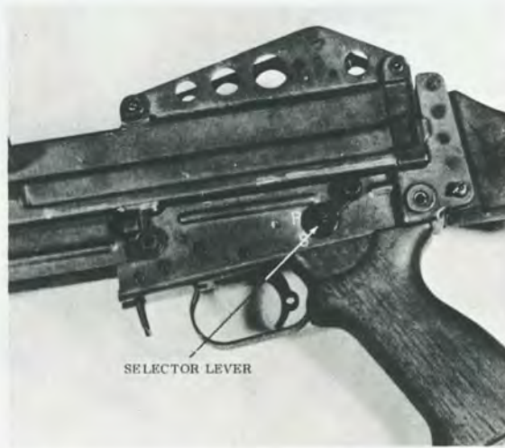
FIGURE 7. — Selector lever on S (safe)
