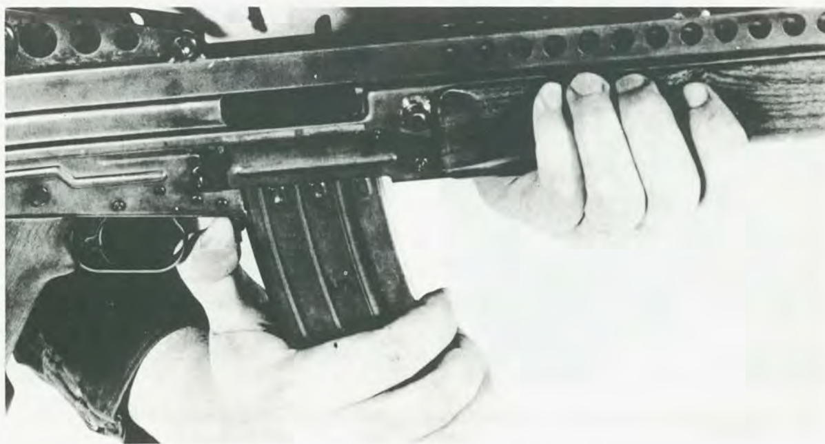
FIGURE 4. — Removing the magazine.
