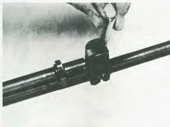
FIGURE 62. — Front sight adjustment.
