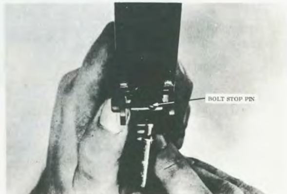
FIGURE 40. — Pushing out the bolt stop pin.
