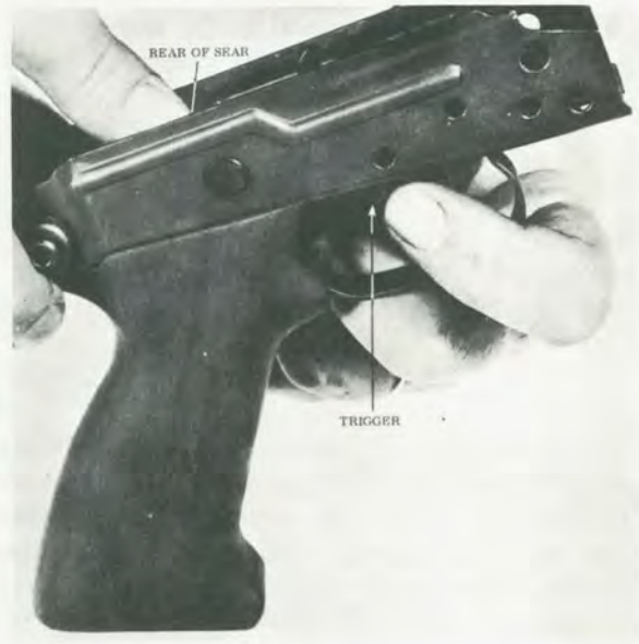
FIGURE 36. — Removing the trigger assembly.
